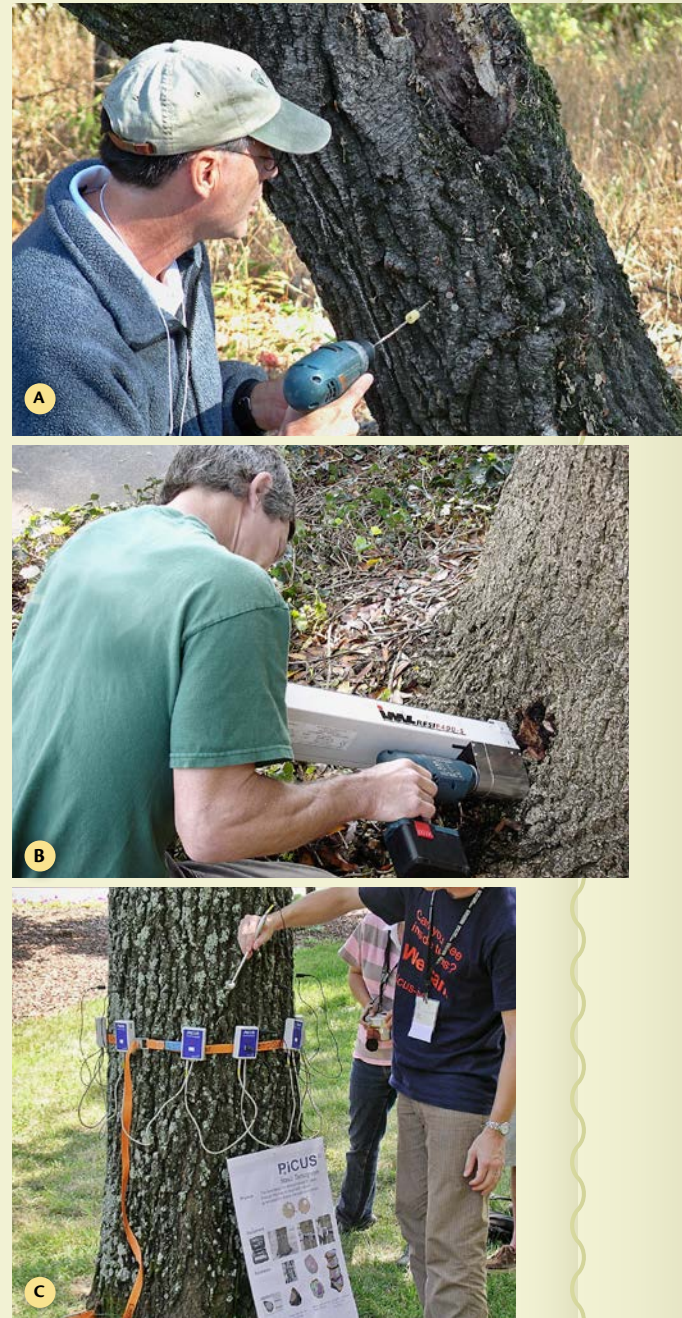
Figure 8.9. Portable drill (A), resistance microdrilling (B), and sonic tomography (C) can be used to determine the extent of decay in oaks. K. JONES
